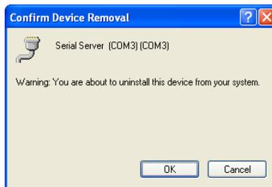
4. The STM-501C COM # will be removed and the Device Manager window will refresh and display the remaining COM ports.
